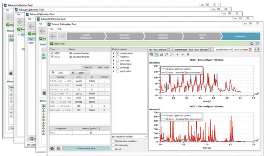
In extreme cases, using a fixed time step solvers of 0.1s, we can execute the simulation of an exhaust after-treatment device over a complete driving cycle in seconds, making it possible to simulate thousands of cycles in a couple of hours.
